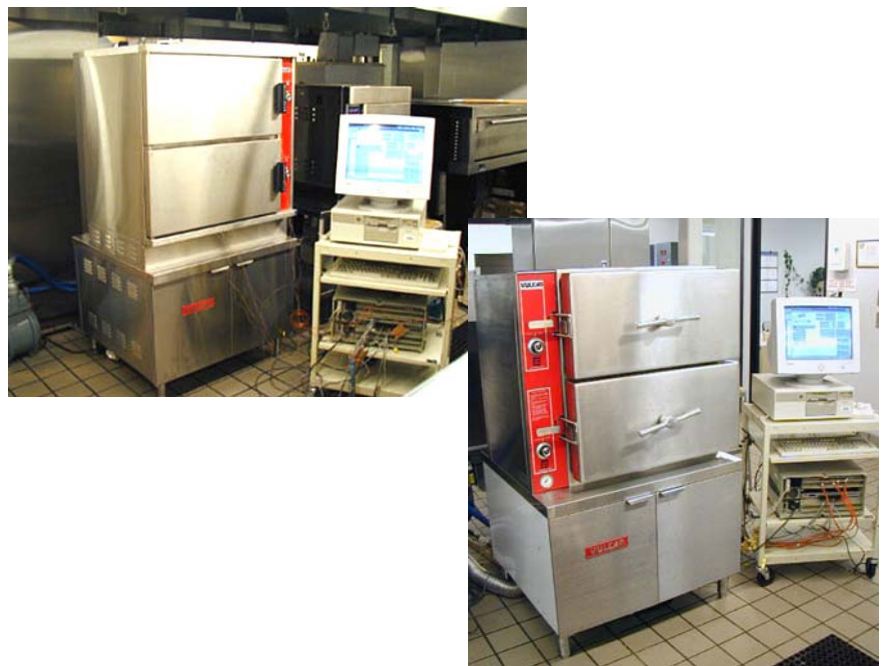
Figure 2-1. The Vulcan VL2GSS and VS3616G Steamers Instru- mented for Testing.
