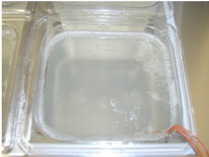
Figure 3. Well with METHOCEL ® K4M slurry and thermocouple.
