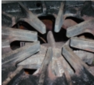
Figure 1-1. Star burner – rated at 20,000 Btu/hr.
