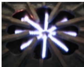
Figure ES-1. Star burner – rated at 20,000 Btu/hr.
