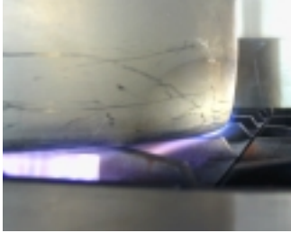
Figure ES-3. A 12" stockpot allowing flames to leak out from the bottom.
