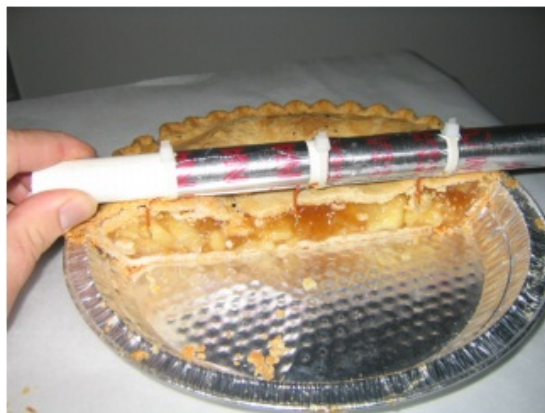
Figure 7: Thermocouple Rig for Measuring Baked Pie Temperature
