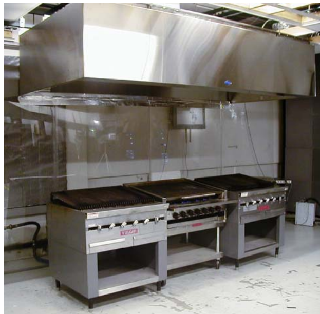
Figure 1. Gaylord PG-ND-BDL-54 Wall-Mounted Canopy Hood Test Setup (Note Transparent Back Wall)
