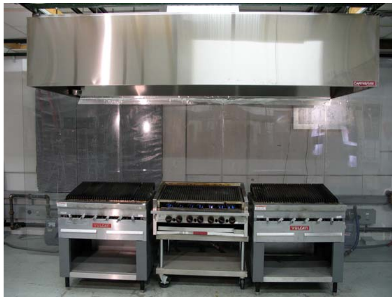
Figure 5. Heavy-Duty Underfired Gas Broiler Line
