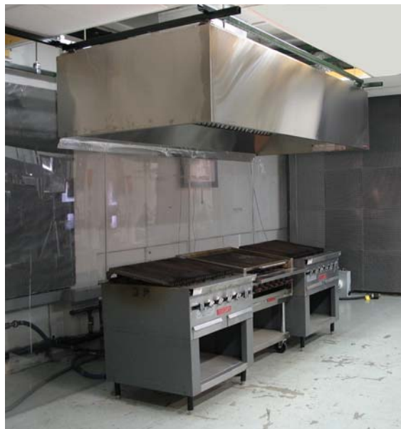
Figure 1. Captive-Aire 5424ND2 Wall-Mounted Canopy Hood Setup (Note Transparent Back Wall)
