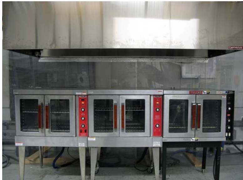
Figure 7. Light-Duty Full Size Convection Oven Line
