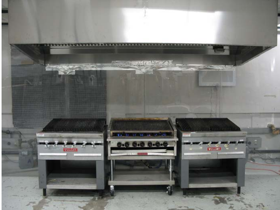
Figure 1. Accurex XXEW-10.0-S Tapered Wall-Mounted Canopy Hood Test Setup (Note Transparent Back Wall)
