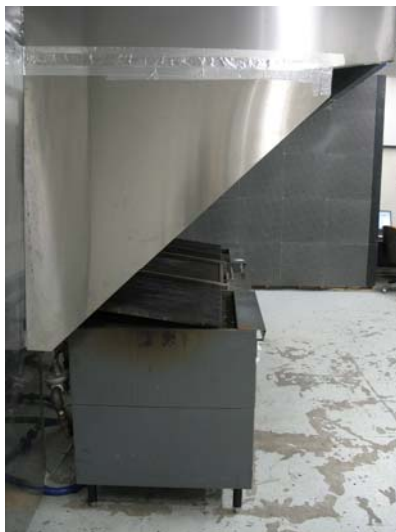
Figure 4. Side View of Set Up With Standard 45-inch by 45-inch by 45° Side Panels
