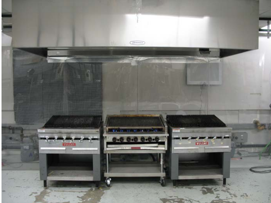
Figure 1. Accurex XXEW-10.0 Wall-Mounted Canopy Hood Test Setup (Note Transparent Back Wall)
