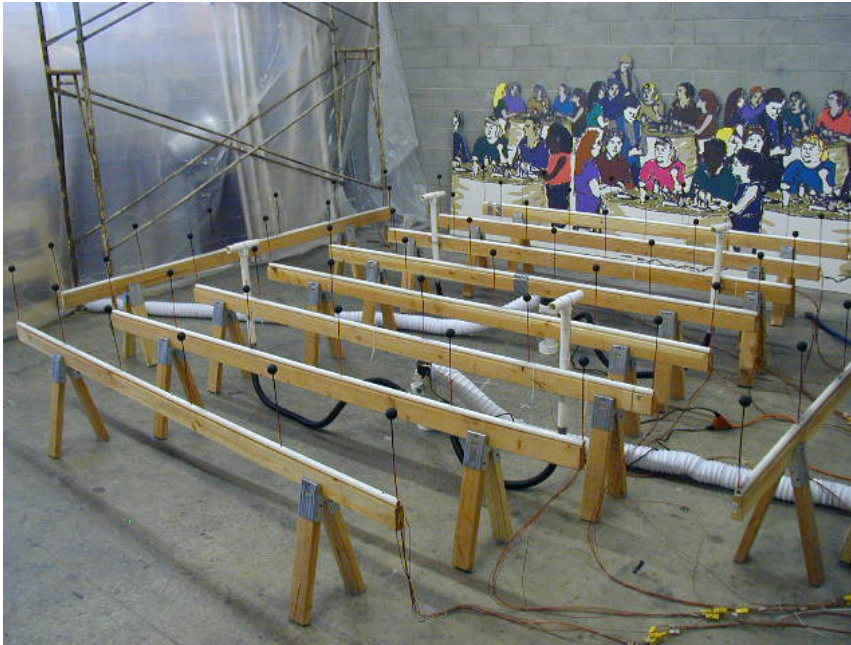
Figure 1. Globe thermometer array.
