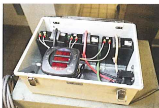
The Comprehensive Commercial Kitchen Equipment Retrofit Project starts by placing submeters on pieces of foodservice equipment to establish baselines for energy consumption.
